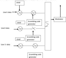
Fig.2 W-CDMATransmission Module
